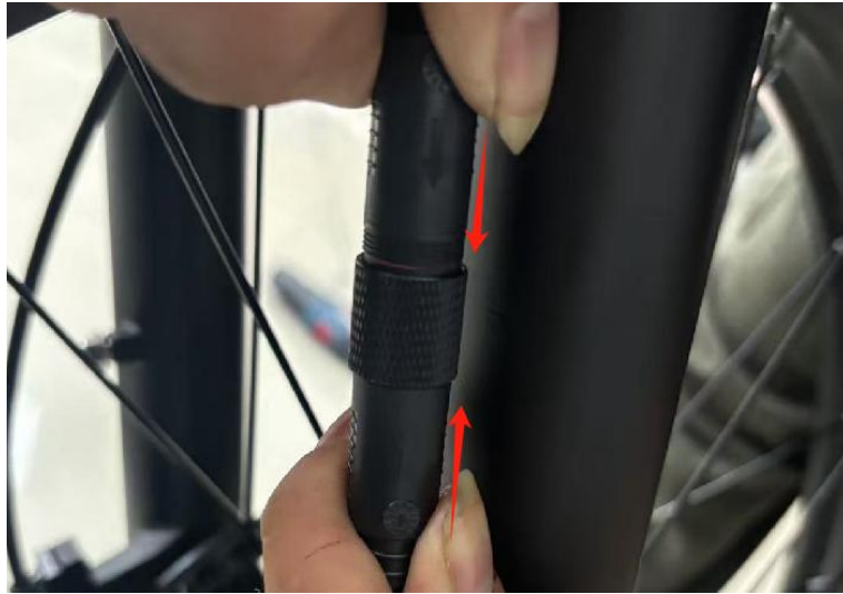
A17.The front motor line should be arrow-aligned
