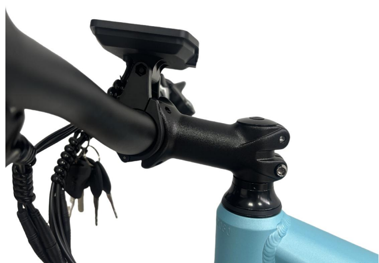
A8. Fit the stem and handlebar together
