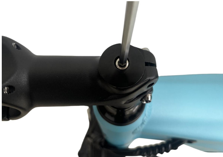
A11. Tighten the top bolt
