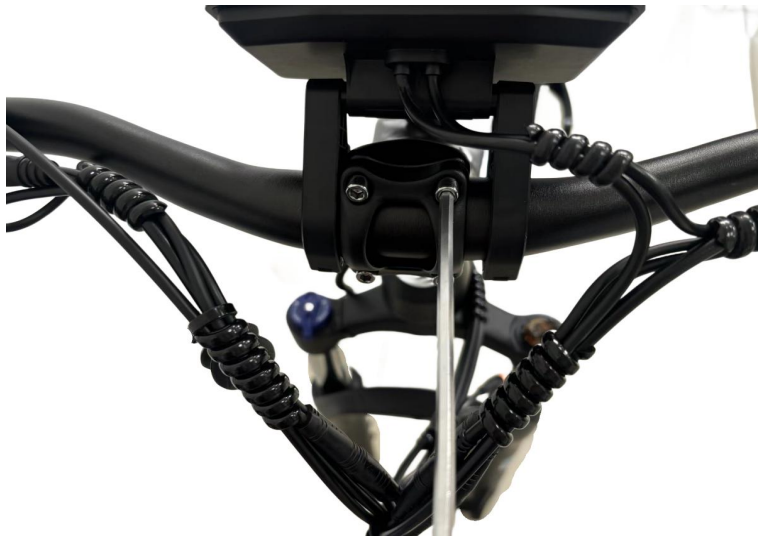
A9. Tighten the 4 bolts to fix handlebar
