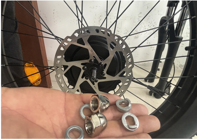
A13.Remove the front wheel screws
