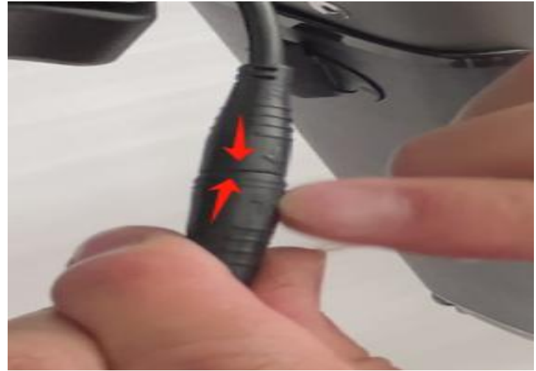
A22.Headlight connection method→ ←, Yellow for headlights
