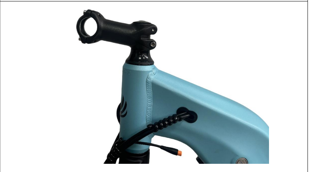
A04. Turn the stem forward ( do not turn the whole fork )
